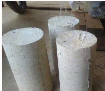
**Gambar 1.** Sampel Benda Uji Beton
