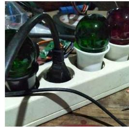
**Gambar 12. Stop Kontak Yang Diberi Beban Mati, Berarti Relay OFF**
