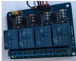
**Gambar 2. Relay Shield**
