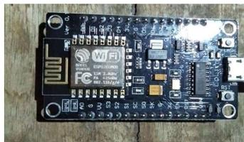
**Gambar 3. NodeMCU ESP8266**
