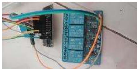
Gambar 13. Rangkaian Relay ke masing-masing channel
