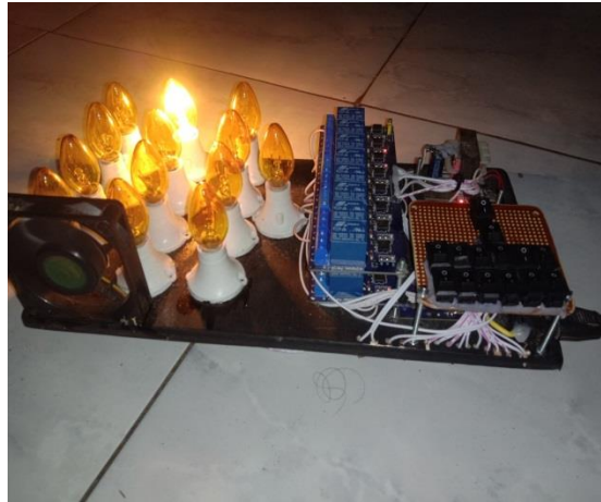
Gambar 10. Pengujian saklar bypass
