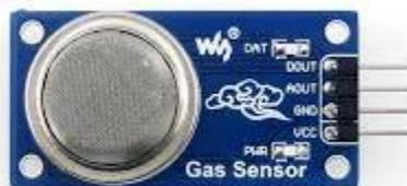
Gambar 2. Modul Sensor MQ-135
